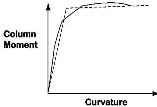
Figure 4.3-3 Typical Moment-Curvature Curve for a Concrete Column
