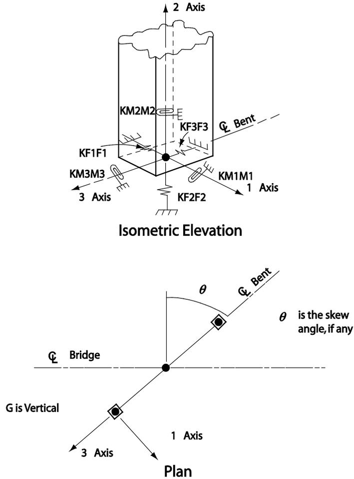
Figure 4.2-9 Foundation Spring Definition at a Bent
