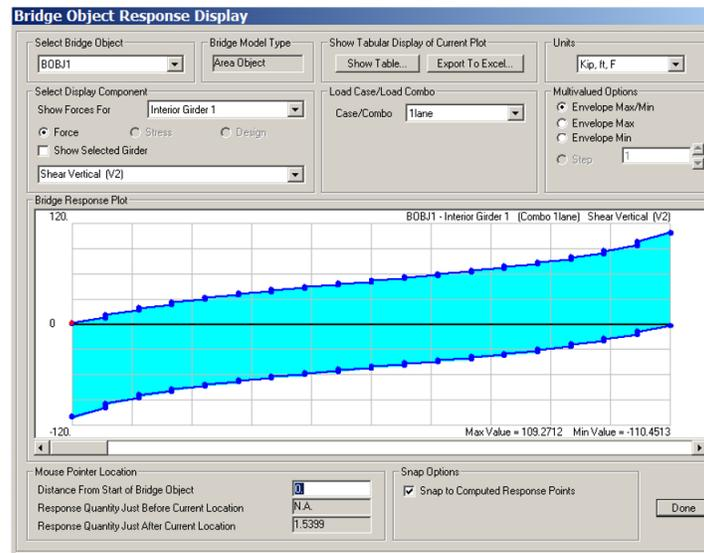
Shear at Interior Girder = 109 Kips at  $x = 0$
