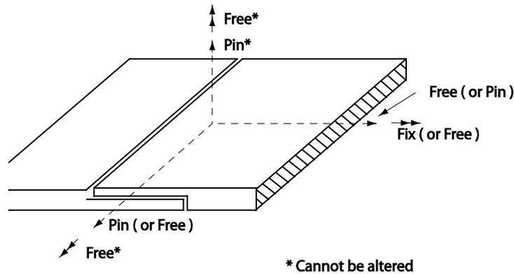
Figure 4.2-7 Span Hinge Force Definitions (Priestley et al, 1996)
