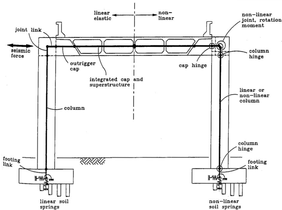
Figure 4.2-8 Multi-Column Bent Model (Priestley et al, 1996)
