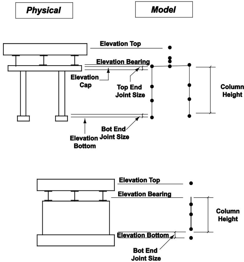
Figure 4.2-6 Superstructure-Bent Connection
