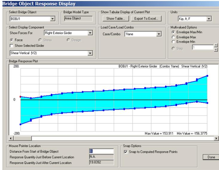
Shear at Right Exterior girder = 154 Kips at x = 0
