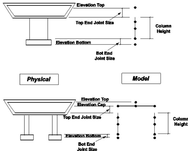
Figure 4.2-2 Model Discretization for Monolithic Connection
