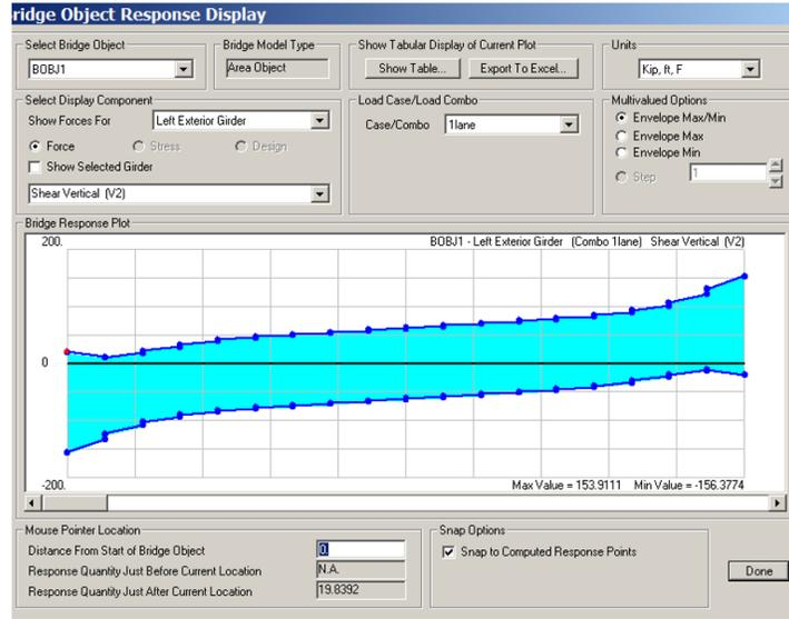
Shear at Left Exterior girder = 154 Kips at  $x = 0$
