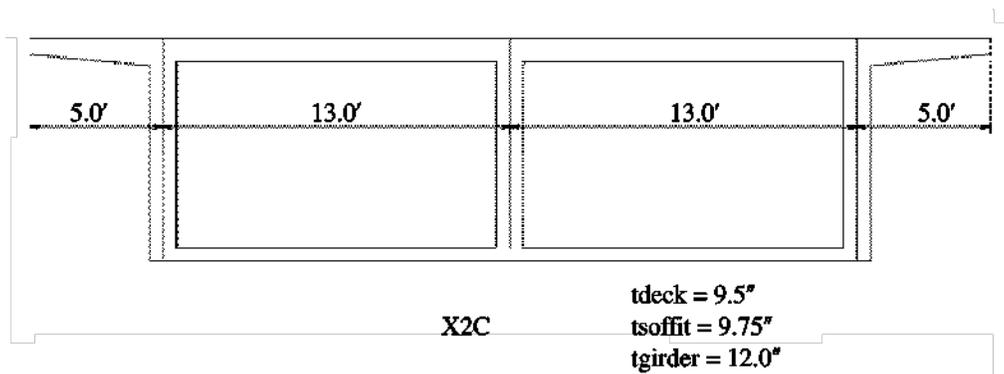
**Figure 4.4-2 Live Load Distribution For Two-Cell Box Girders Snapshot**
