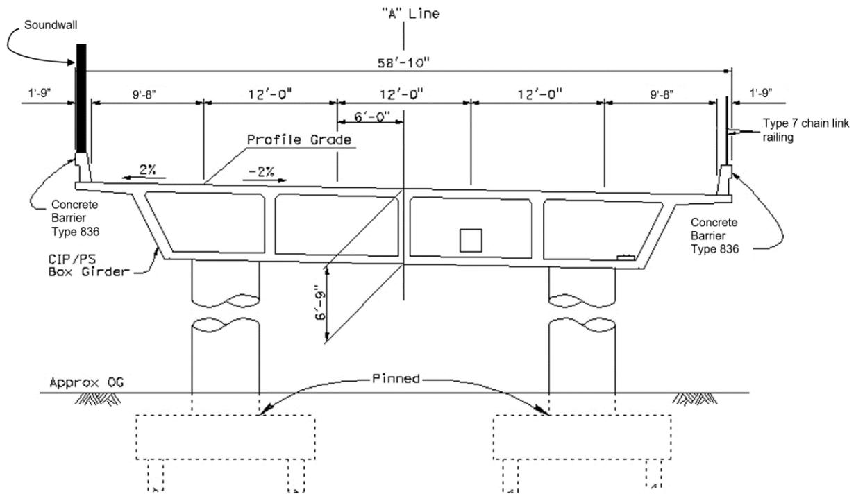
Figure 4.2-13b Typical Section View of Example Bridge
