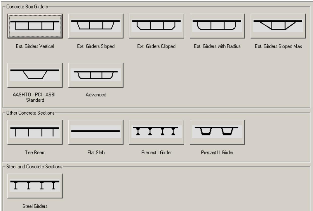
**Figure 4.2-17 Various Bridge Sections**
