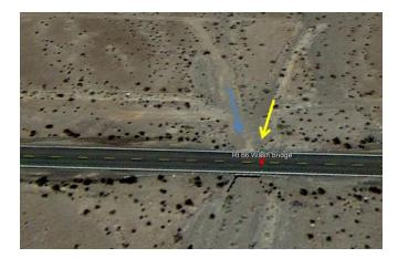
Figure B2.10. Stream crossing alignment with upstream flow in main channel (yellow arrow) complicated by tributary gully (blue arrow), unnamed wash 3.5 miles east of Ludlow, California. Looking upstream.
