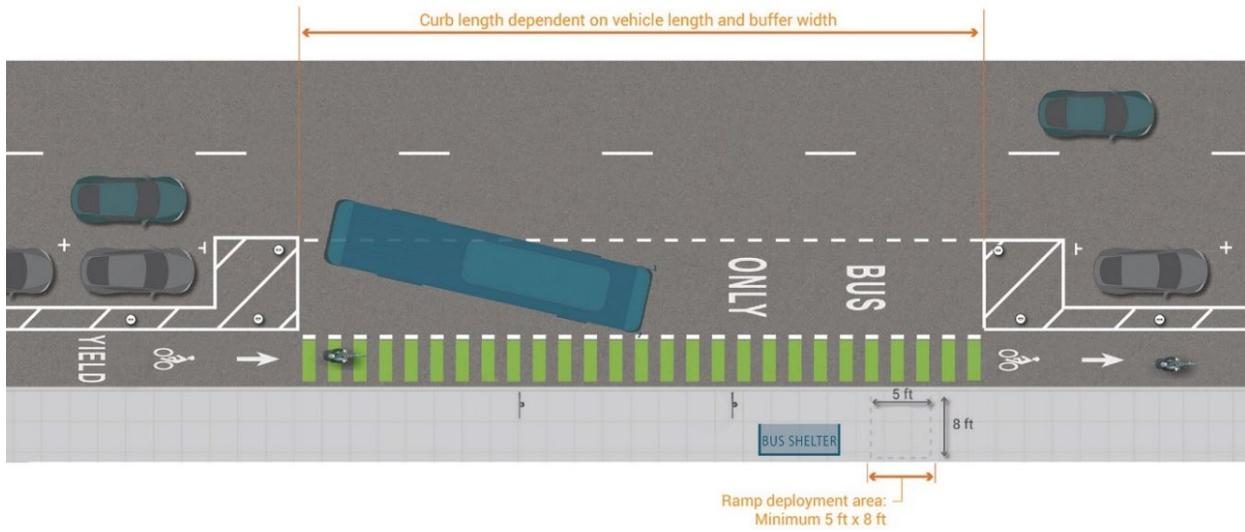
**Figure 7-I - Example of bikeway markings at a bus stop and Bus Only lane in San Francisco**
