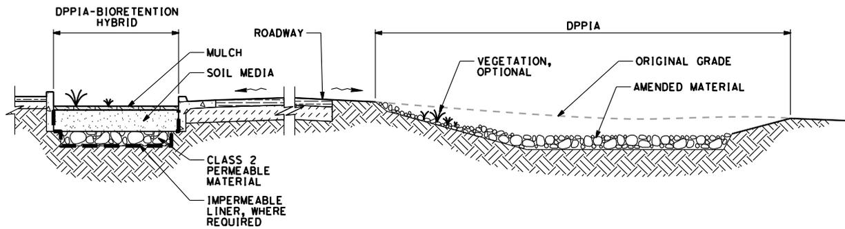
Figure 8-I – Example Detention Basin Treatment BMP
