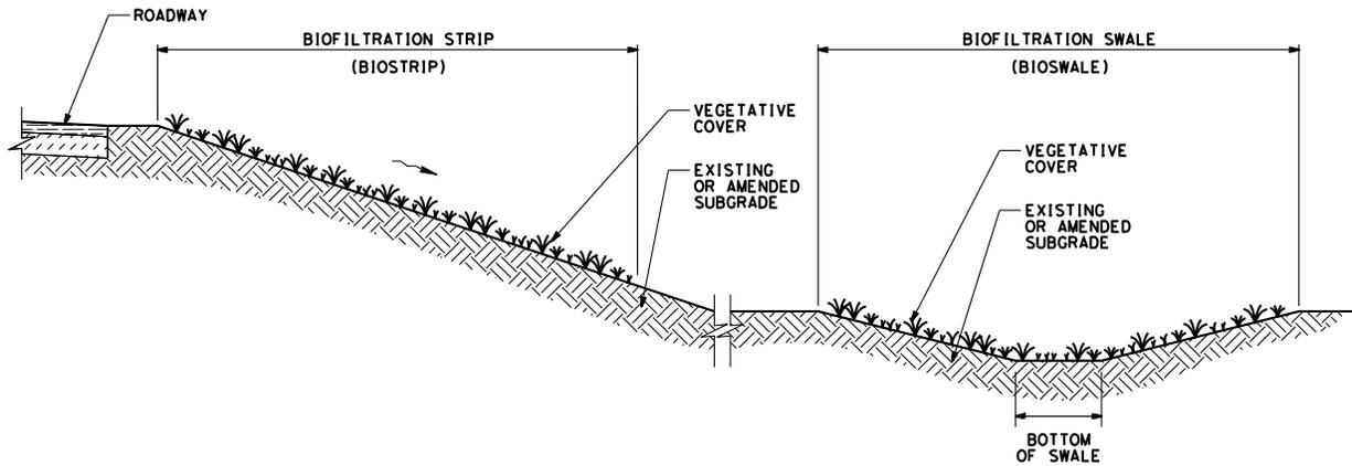
Figure 8-H – Example Design Pollution Prevention Infiltration Area Treatment BMP
