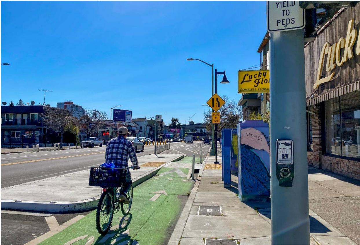
**Figure 7-F - Bus boarding island integrated with parking separation in Berkeley**
