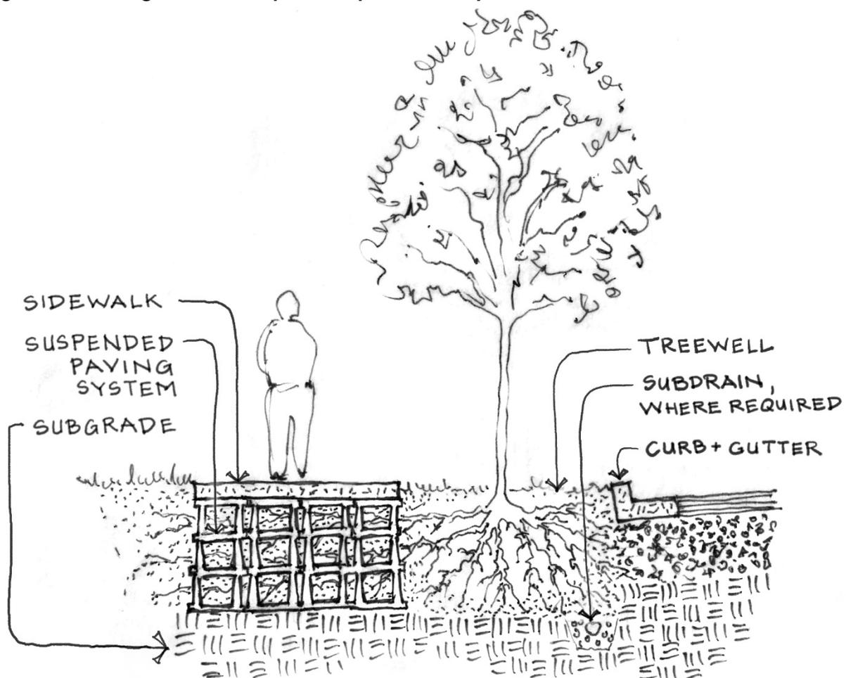
**Figure 8-E – Diagram of a structural soil system**
