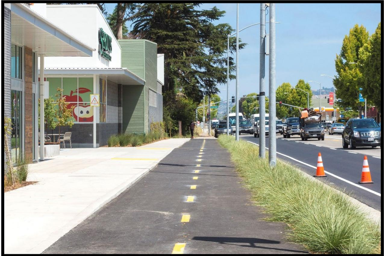
**Photo 9: Two-way Separated Bikeway with pedestrian path grade separation**
