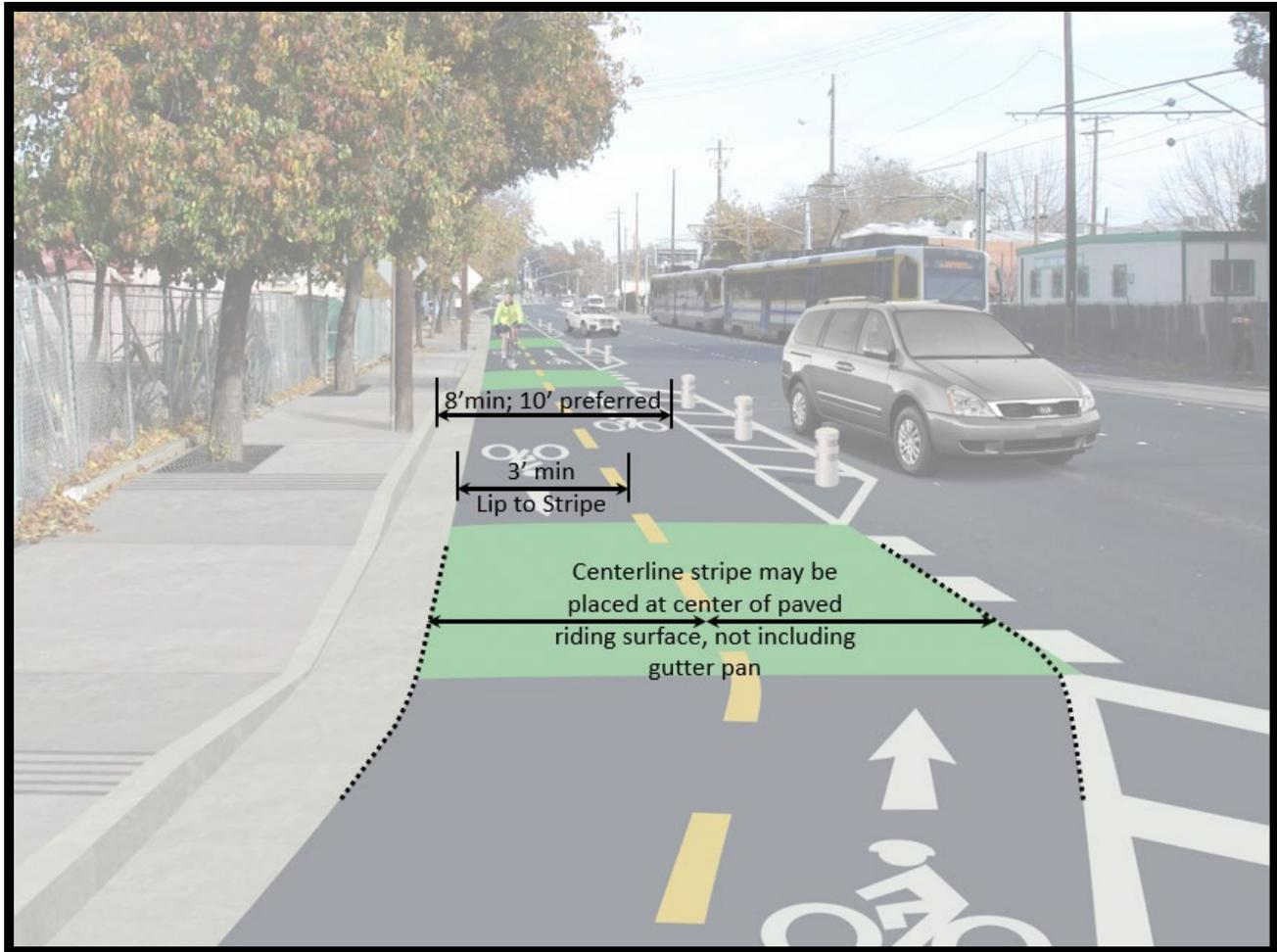
**Photo 10: Two-Way Class IV Bikeway Dimensions (Image Source: Psomas)**
