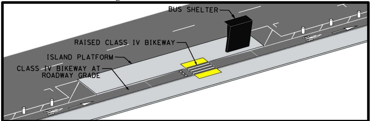
**Figure 3: Busbay Island Platform**
