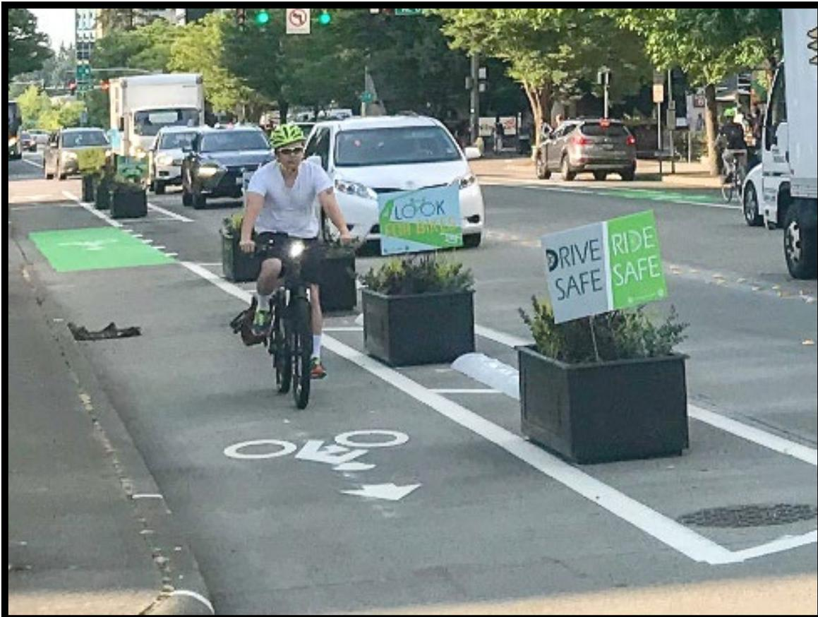
**Photo 11: Separated Bikeway with planters (Image source: City of Bellevue, Washington)**
