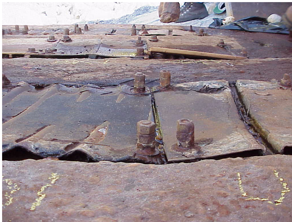
Various Culvert Material Test Panels Shown Above After 1 Year Of Wear At Site With Moderate To Severe Abrasion (Velocities Generally Exceed 10 ft/s, See Table Next Page). Note: the significant wear to abrasive resistant protective coatings, which, would typically not be recommended under these conditions (see table next page). The bed load material composed of 90% quartz sand. Also note the wear on the leading edges (right) of the steel nuts.
