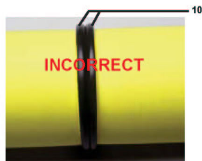
10. Excessive heat time or pressure applied during heating; melt bead too large
