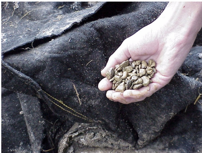
Non-Woven Polypropylene Geotextile Material and 3/8” – 3/4” inch Diameter Gravel from Gravel Bag Headwall Used to Make Filters
