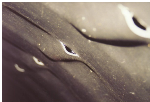
Splitting of 60 inch Diameter Pipe. This Pipe was Installed in 1996 by Another State
