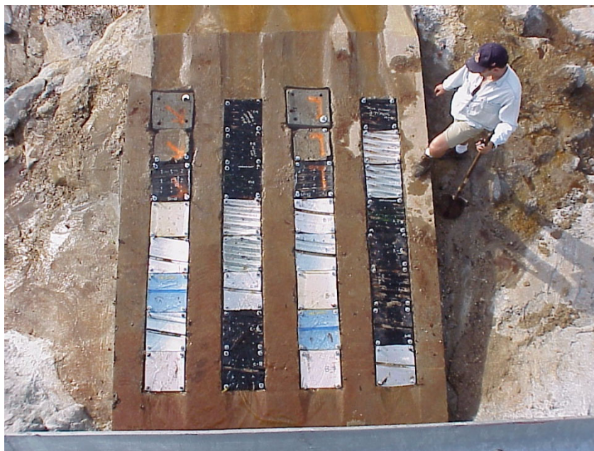
Caltrans Abrasion Test Panel Installation Showing Various Culvert Materials and Coatings
