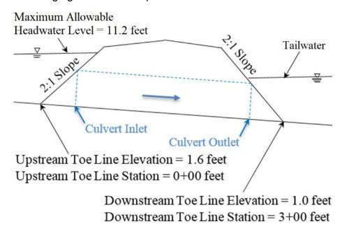
Step 1: Obtain the Tailwater Depth for the corresponding discharge to represent a 1% probability of exceedance event.
