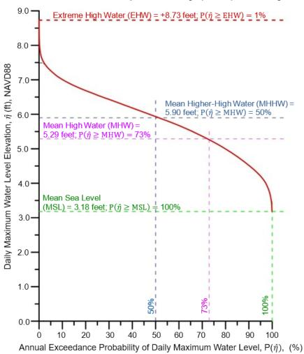
For instance, when determining the backwater effect by a hydraulic structure near outer San Francisco Bay, any of the following pairs of boundary conditions obtained from Figure 821.1 would represent the compound probability exceedance of 1%:
