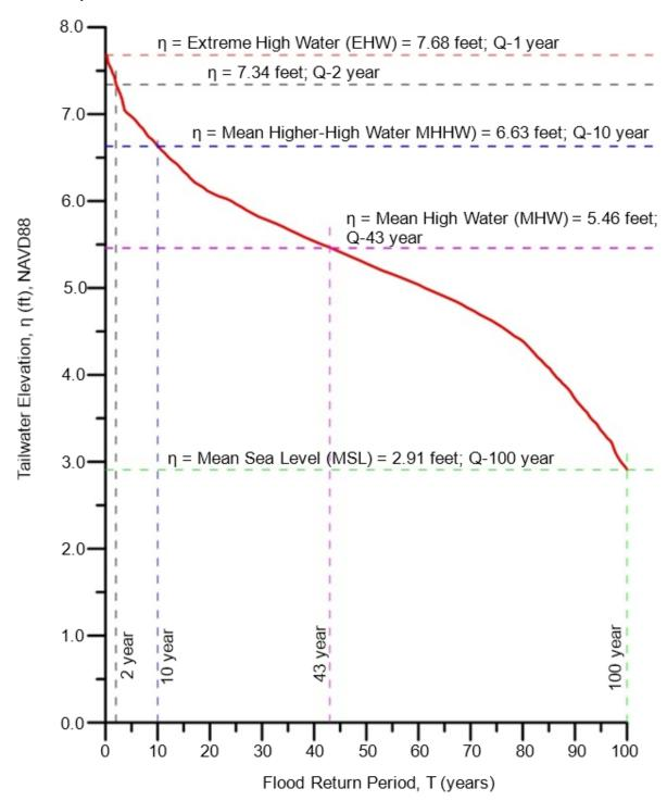
The following provides guidance on how the tailwater level at a project location can be determined based on the one-percent compound frequency curves described above. Let us consider, Province A and Province B are two neighboring provinces, and the distance from the centroid of the province to the boundary is  $L_A$  and  $L_B$ , respectively, as shown in Figure 821.4. The project site is located at a distance  $X_A$  from the boundary within Province A.
