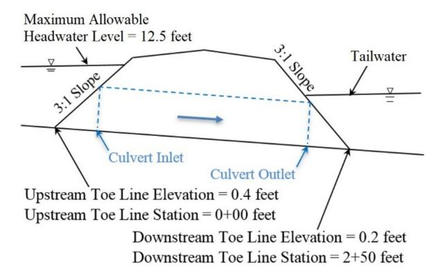
Step 1: Obtain the Tailwater Depth for the corresponding discharge to represent a 1% probability of exceedance event
