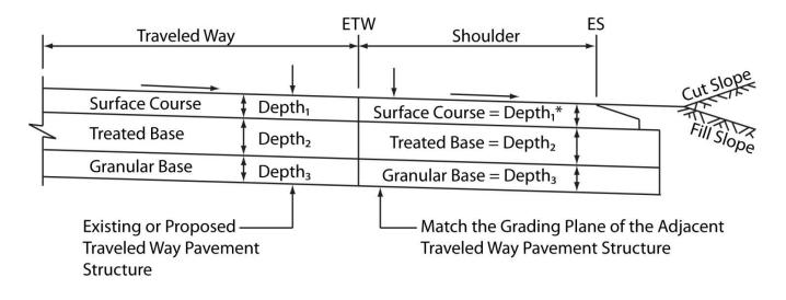
Variable Shoulder Thickness Option for Asphalt Pavement
