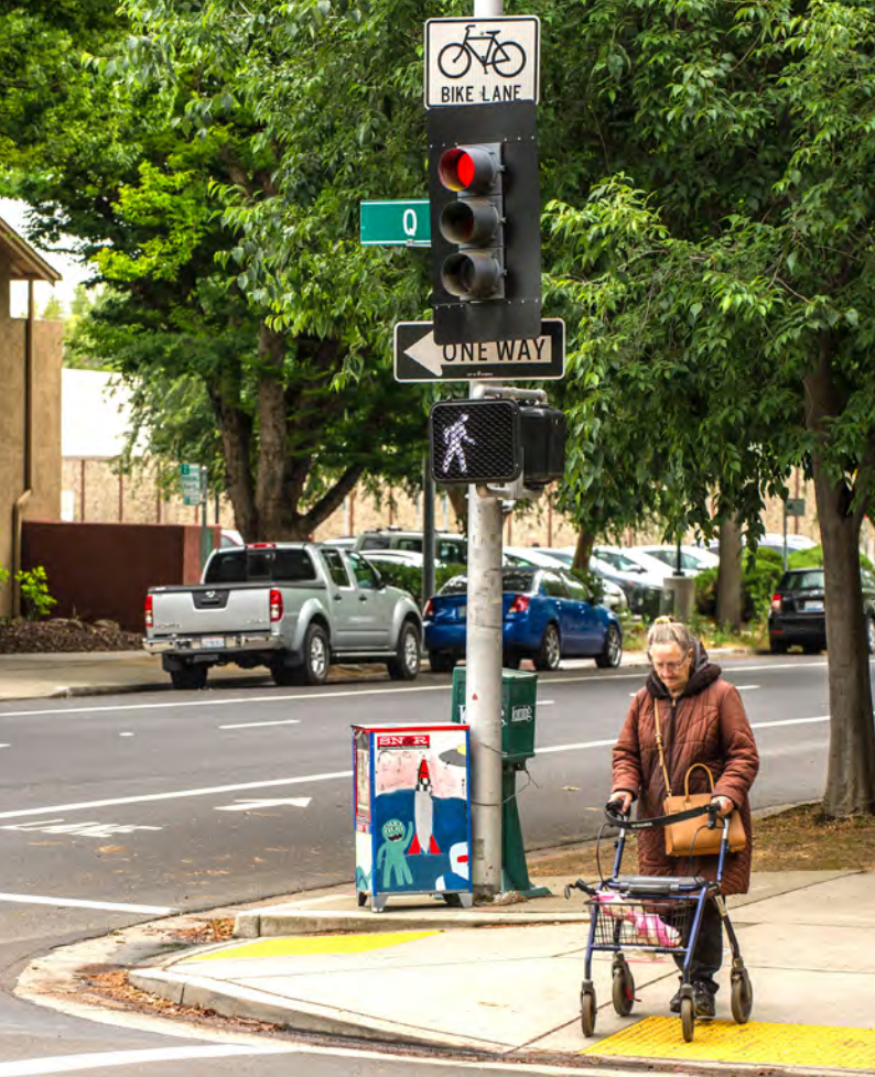
A Leading Pedestrian Interval enables a pedestrian to begin crossing before the parallel traffic gets a green light in Sacramento
