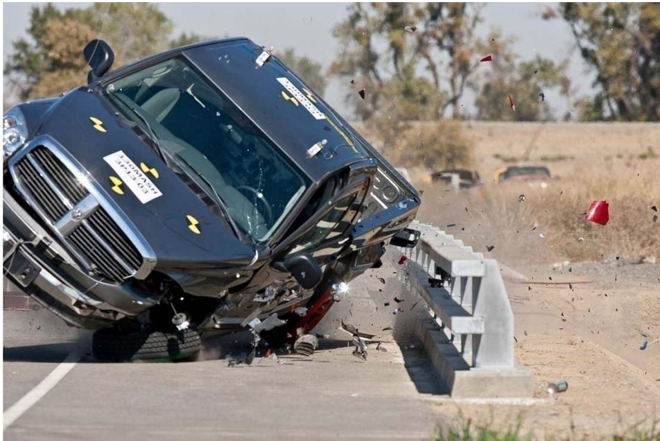
Figure 5-9 Vehicle Riding on Drive Side Front Tire
