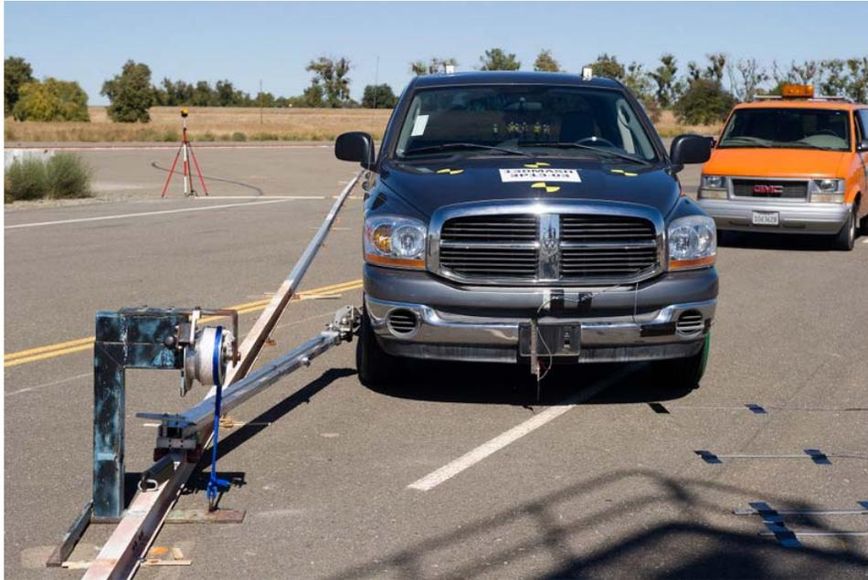
Figure 4-2 Guidance Arm Release Mechanism
