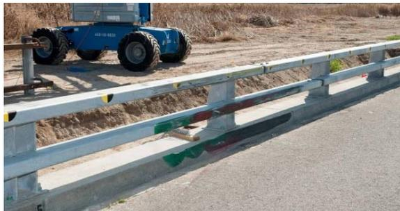
**Figure 5 – Damage to Test Article**
