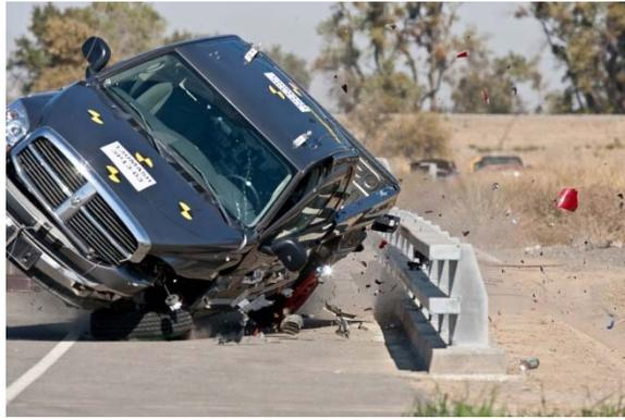
**Figure 2 – Vehicle Impacting the Test Article**
