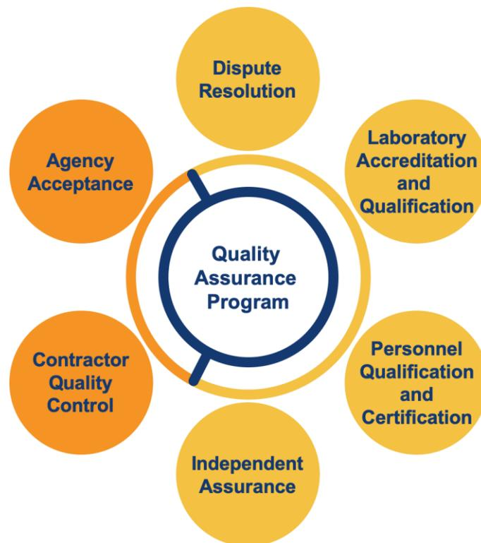
Figure 1. FHWA Six Core Elements of Quality Assurance Program
