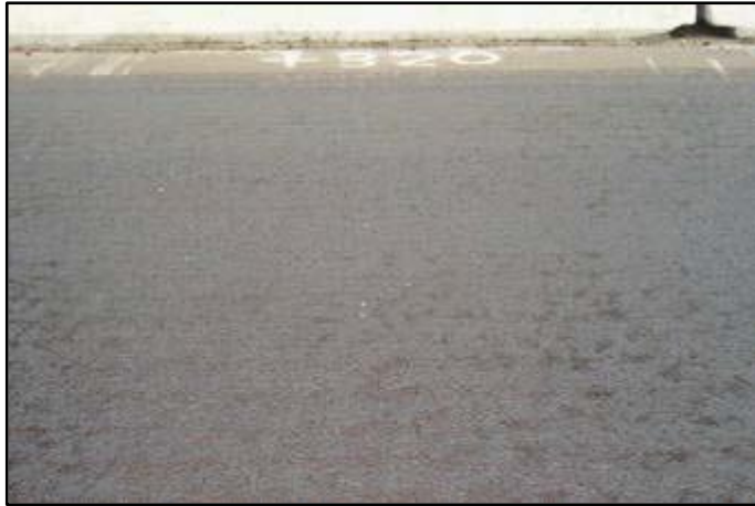
Figure 8-8. The same tack coat 23 minutes later. The brown color now appears in splotches, indicating it is beginning to break.
