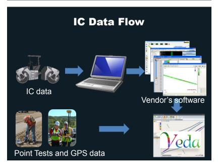
Intelligent Compaction is also used to map the stiffness of the underlying material in order to establish the baseline stiffness of the materials and to identify areas of weak support. On a new construction project, mapping will be conducted on the in-place materials (soils and/or aggregate) base materials. Where an HMA overlay is being placed over an existing asphalt pavement, mapping will be conducted on the existing asphalt pavement or on the pavement after milling operations are completed.
