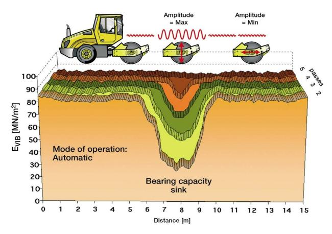
Although there are efforts to use Intelligent Compaction as an acceptance tool, however at this time, Intelligent Compaction is being used as a quality control tool helping contractors to achieve uniform compaction by monitoring the rolling pattern, temperature and stiffness.
