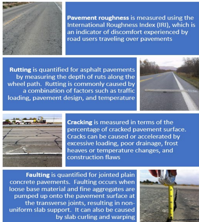
Figure 5-6. Examples of Pavement Conditions
