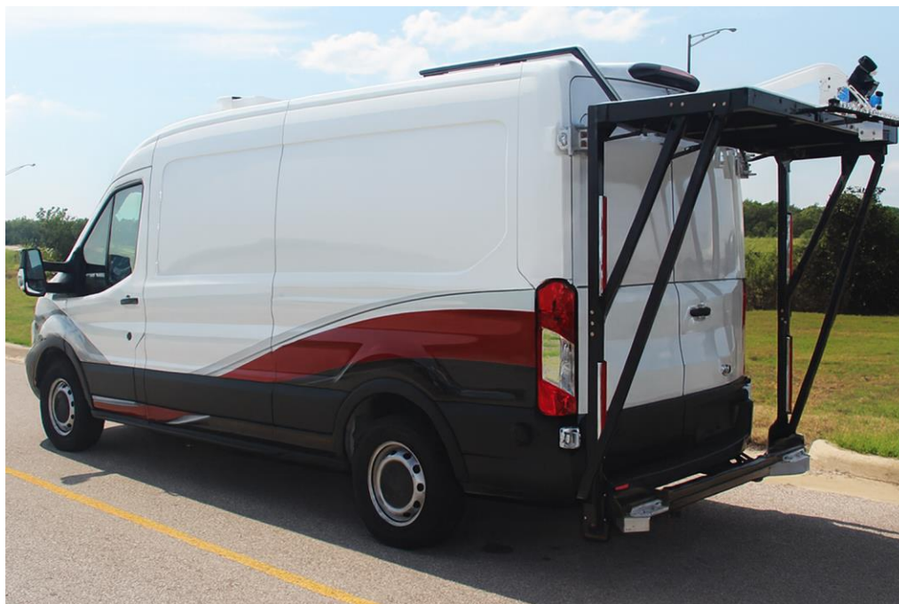
Figure 4-4. Automated Pavement Condition Survey Vehicle
