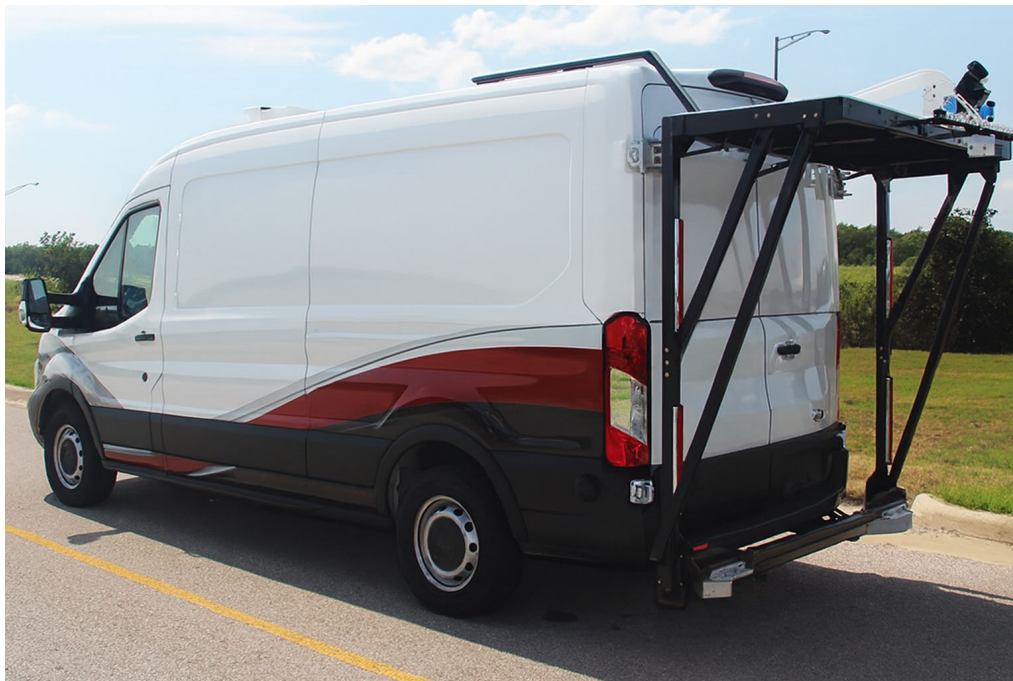
Figure 4-4. Automated Pavement Condition Survey Vehicle
