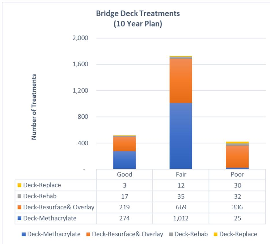
Figure 4-6. Bridge Deck Treatments (10 Year Plan)
