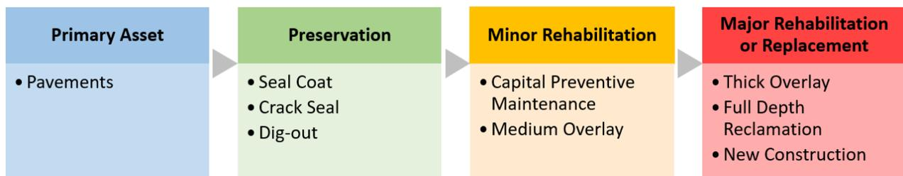
Figure 6-2. Typical Asphalt Pavement Life Cycle Planning Treatments
