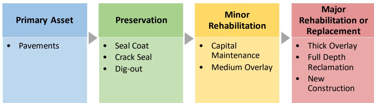
Figure 6-2. Typical Asphalt Pavement Life Cycle Planning Treatments
