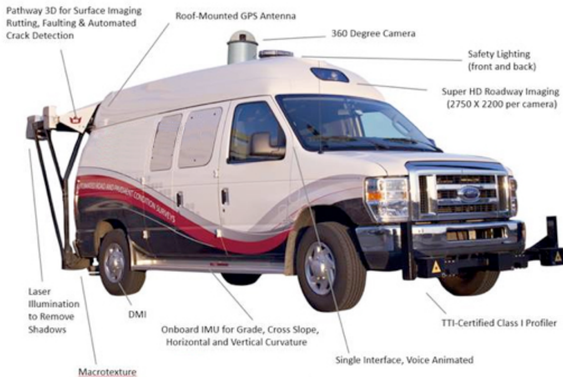
Figure 4-3. Automated Road and Pavement Condition Survey Van
