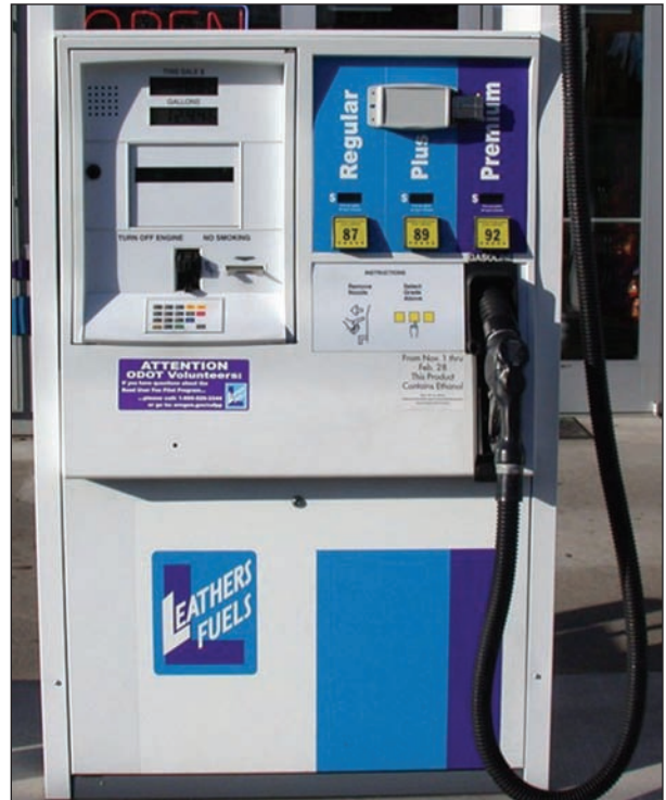
Figure 3. Wireless receiver (white box) mounted to fuel pump in Oregon pilot program.
