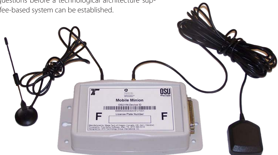
Mileage counter and wireless mileage transmitter utilized in Oregon pilot program.
