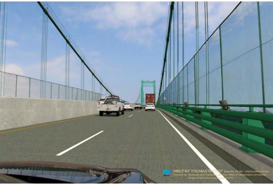
Figure 2.11-8: Photo Simulation of Proposed Bridge Rail (Suspended Span)
