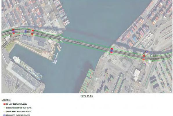
Figure 1-5: Eight Proposed Locations of Bridge Construction Elevators
