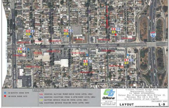
Figure 2.14-47: One Lane Open Each Direction – Sepulveda Blvd
