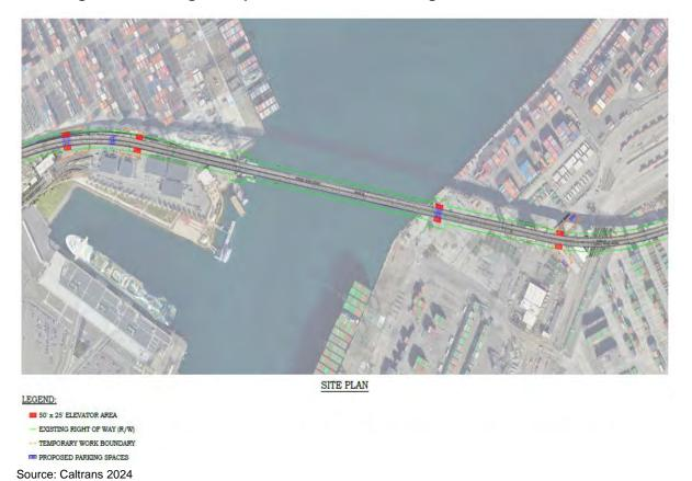
Figure 2.22-2: Eight Proposed Locations of Bridge Construction Elevators
