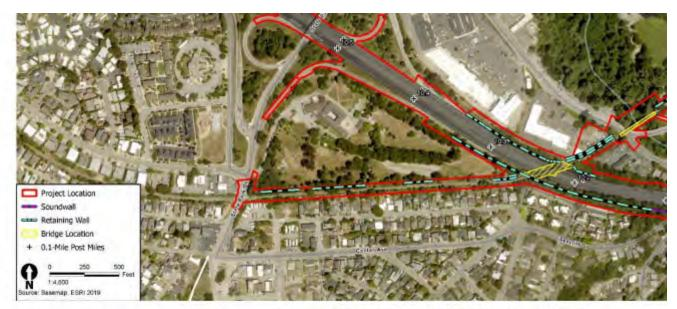
Figure 1-3a. Project Components, Sheet 1 of 3
