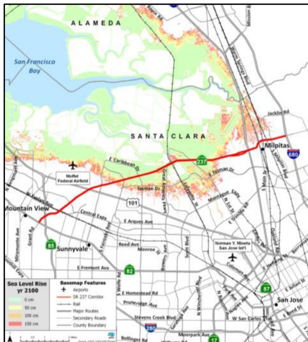
Figure 16. Vulnerable areas of SR 237 currently at risk and at increased risk with further sea-level rise. Source: USGS CASCade Project http://cascade.wr.usgs.gov/data/Task2b-SFBay/index.shtm
