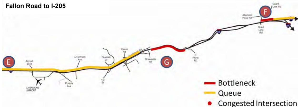
Figure 5: Existing 2008 Recurrent Weekday Congestion on I-580 (from ALA-238/580 Corridor System Management Plan Technical Analysis Report-Volume 1, Section 2, Figure 21, page 69)
