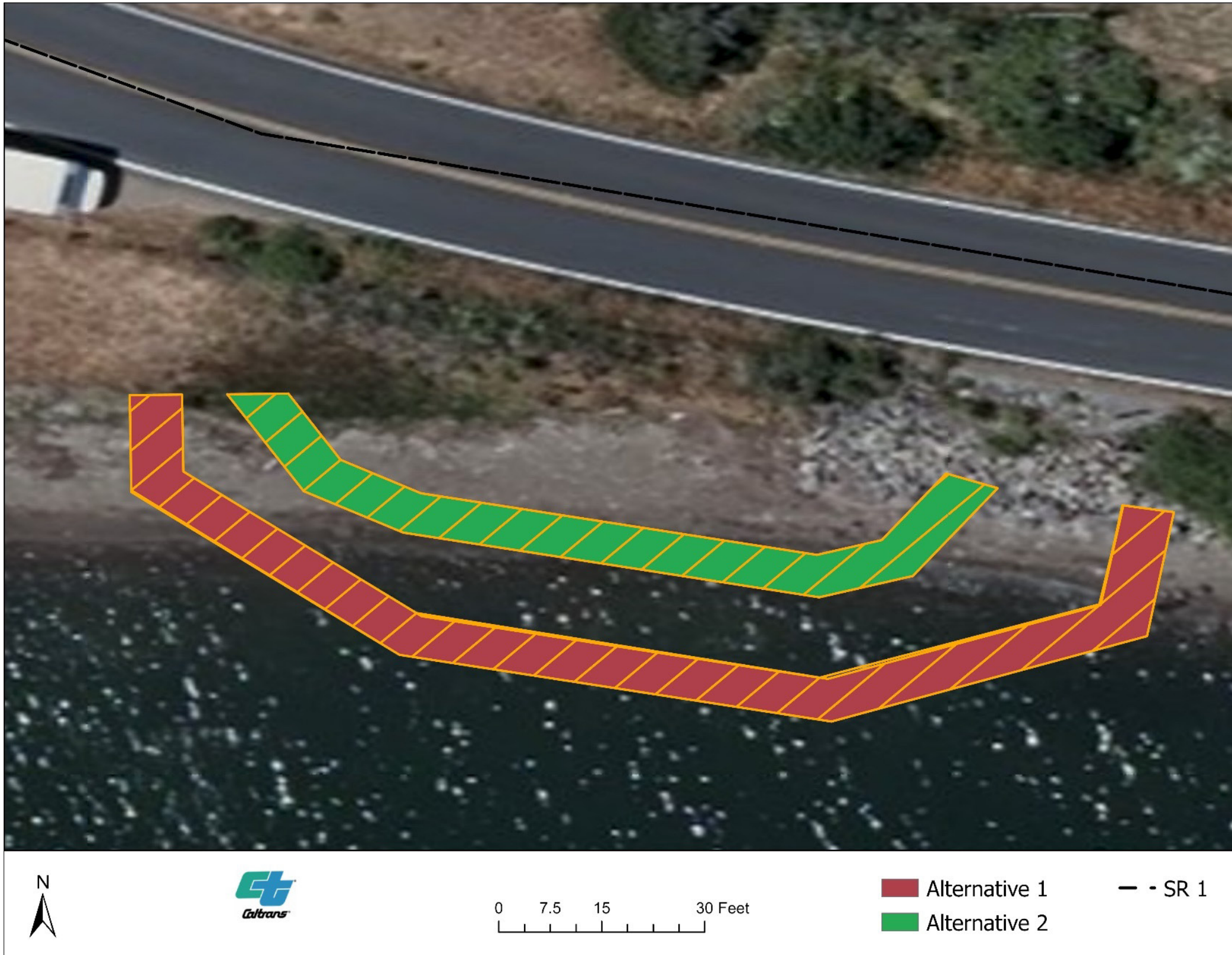
Figure 11. Proposed placement of cofferdams under Alternatives 1 and 2.
