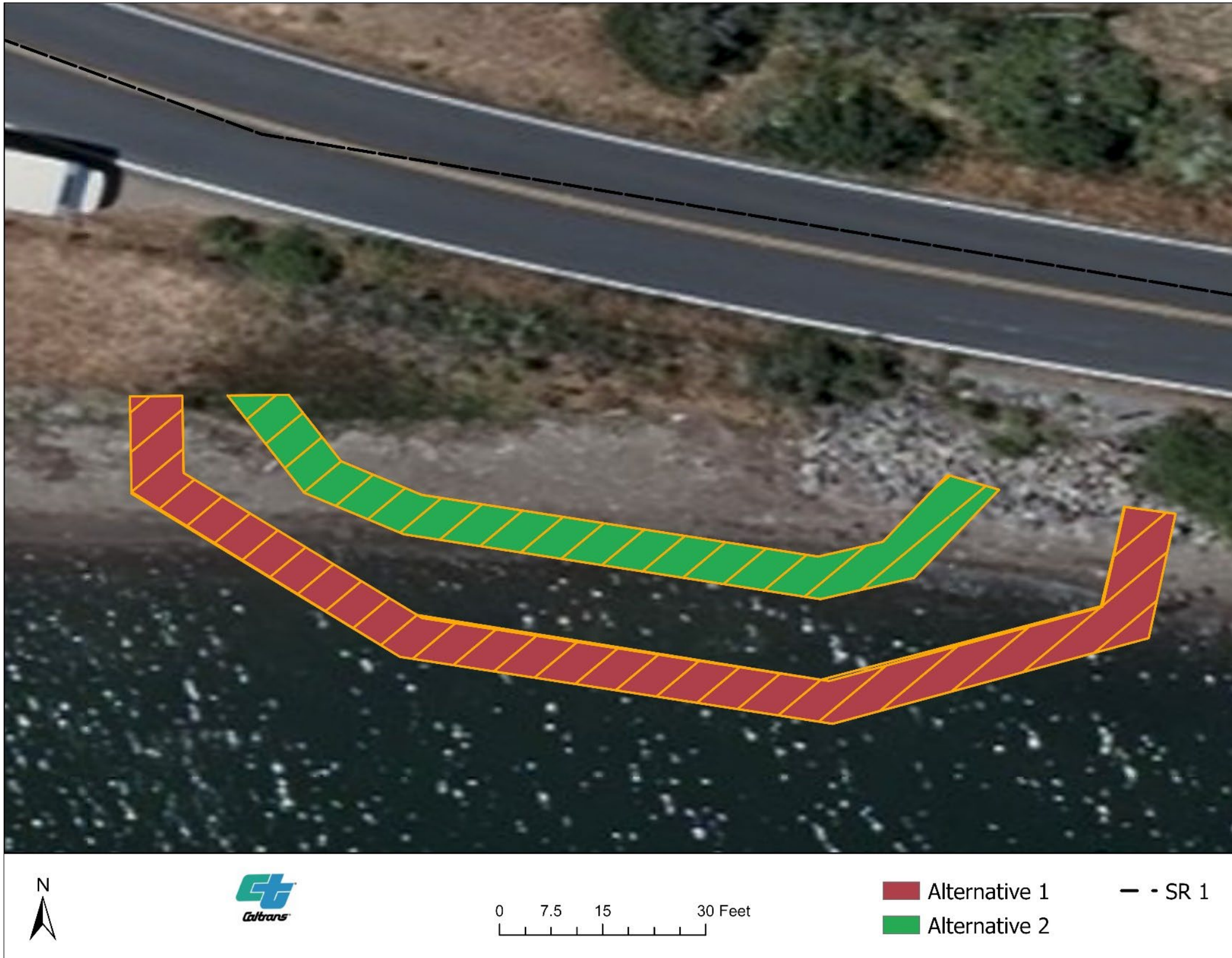
Figure 11. Proposed placement of cofferdams under Alternatives 1 and 2.
