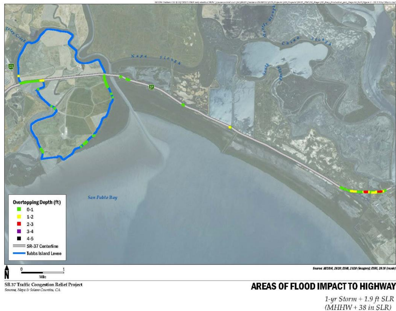
Figure 3-13 Areas of Flood Impact to Highway Under 1.9 Feet of SLR Conditions with a 1-Year Storm Scenario
