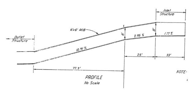
Figure 12. 1917 As-Built Profile of the Fish Creek Culvert
