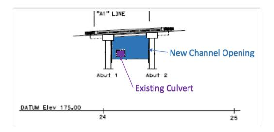
Figure 14. Diagram of new channel opening and existing culvert
