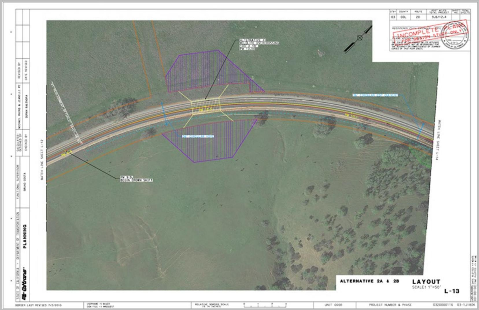
**Appendix Figure 1.** Preliminary scoping map used at the beginning of the design phase. This shows the initial placement of the overcrossing to be used by Caltrans Structures & Design Team as a rough estimate location.
