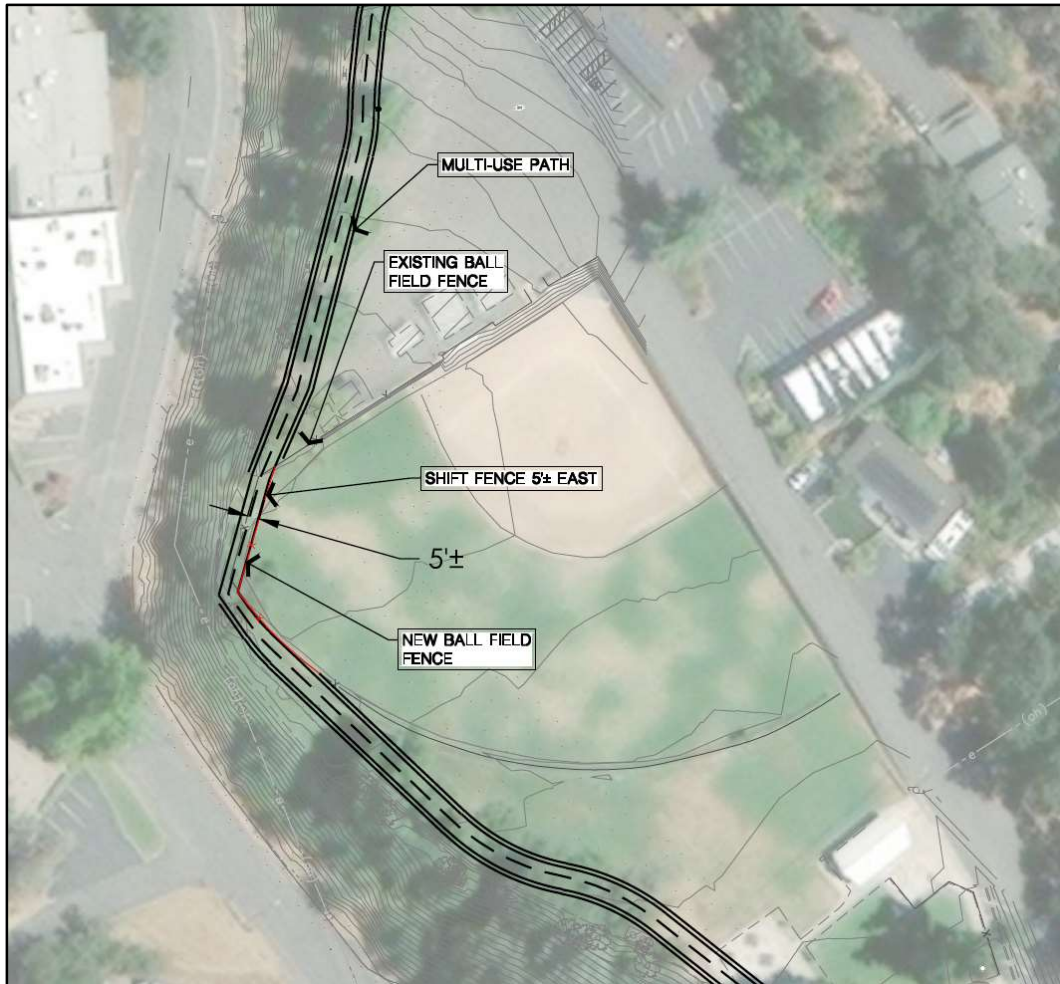
Figure 2. Build Alternative 1 Fence Relocation Concept
