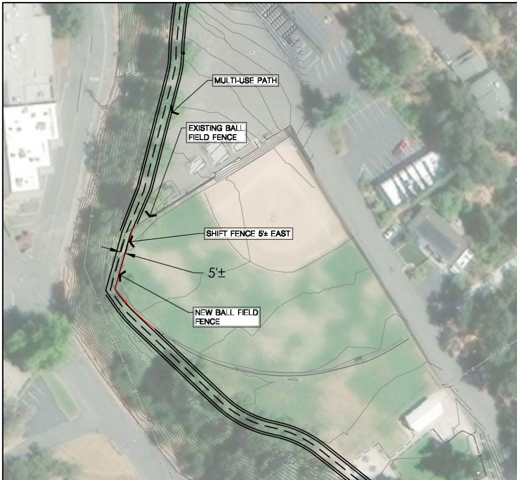
Figure 2. Build Alternative 1 Fence Relocation Concept
