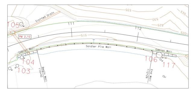
Figure 11. Detail of proposed retaining wall at post mile 2.10 (Yniguez 2015).
