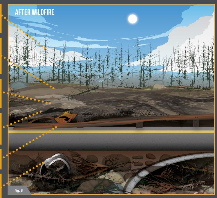
After a wildfire, new risks are posed to transportation assets in the area. Immediately after a fire, the loss of signs and guardrails presents a danger to travelers and require an immediate response. Other impacts noted in the graphic above can exist as a potential risk to Caltrans assets for years after a wildfire event occurs.
