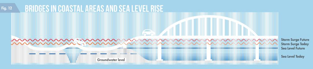
Climate change can impact infrastructure in multiple ways. Bridges in coastal areas, for example, can be directly impacted by rising sea levels and storm surge effects. Today's bridges were designed and built for current tidal and surge conditions, so increasing water levels may increase the risk to these facilities in the future.
