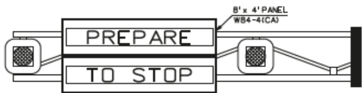
AW-IV: W89(CA) "PREPARE TO STOP" ABO (Overhead Mounted)
