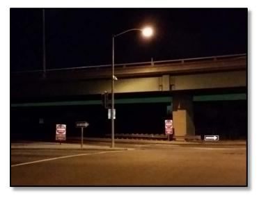
The wrong way packages at these off-ramps, as well as other off-ramps in the Sacramento area, meet or exceed the wrong way sign standards outlined in the California edition of the *Manual of Uniform Traffic Control Devices*. Although the high level of intoxication for each driver undoubtedly contributed to the decision to enter the freeway off-ramp in the wrong direction, reasons why the ramp attracted the inebriated driver is unknown.
