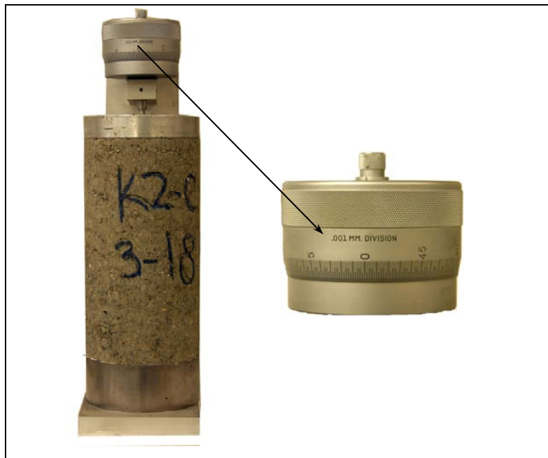
Figure 9.17: Apparatus for measuring shrinkage of cured specimens.
