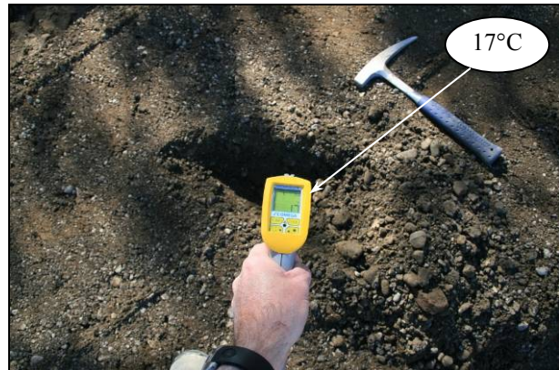
Figure 7.27: Recycled material (cold).
