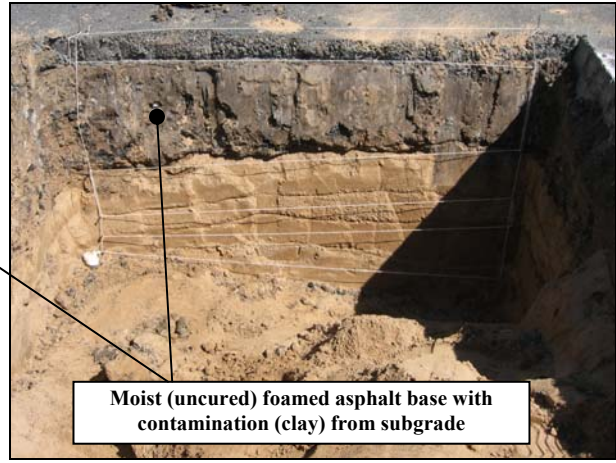
Figure 4.30: Test pit #2 on 05-SB,SLO-33.
