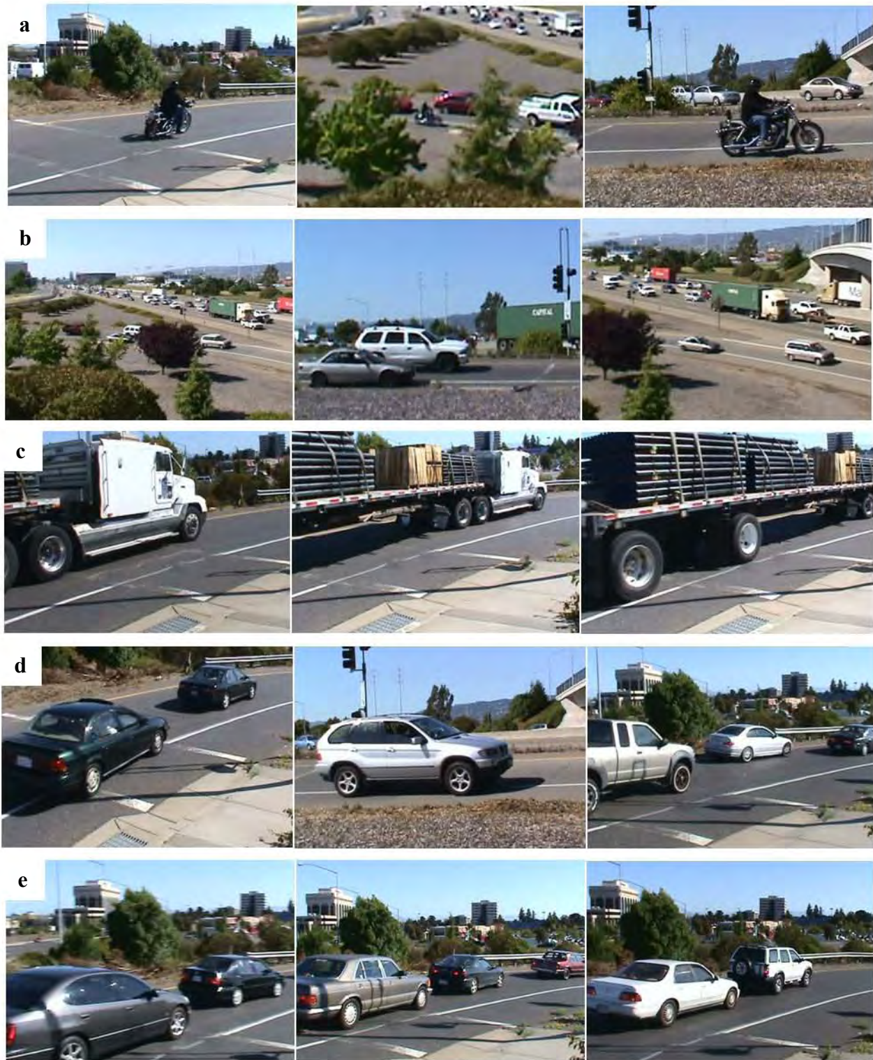
FIGURE 19 (a) Motorcycle bypassing queue. (b) Vehicle bypassing queue. (c) Large truck entering the on-ramp. (d) Off-centered vehicles with respect to the lane. (e) Adjacent vehicles simultaneously stopped on top of the leading and trailing speed trap sensors.
