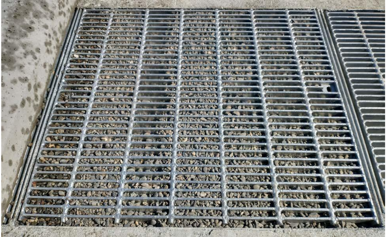
Figure B.3: Test#1 Pass 2 (3/8-inch pea gravel after sweeper pass at very slow speed
