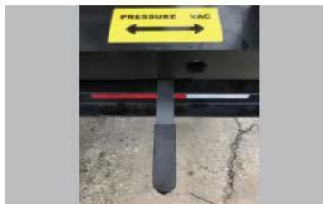
REVERSE PRESSURE. Reverse pressure to offload liquids and dislodge debris in hose.
