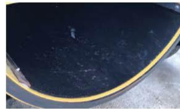
POLYMER LINER. The polymer liner inside the debris tank on the bottom half makes for ease of dumping and cleanout.
