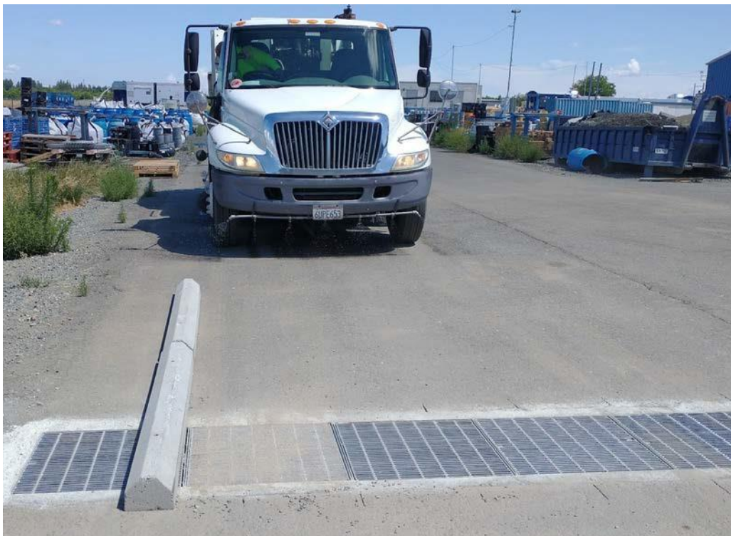
Figure 4.4: Sweeper approaching grate for a test with sand
