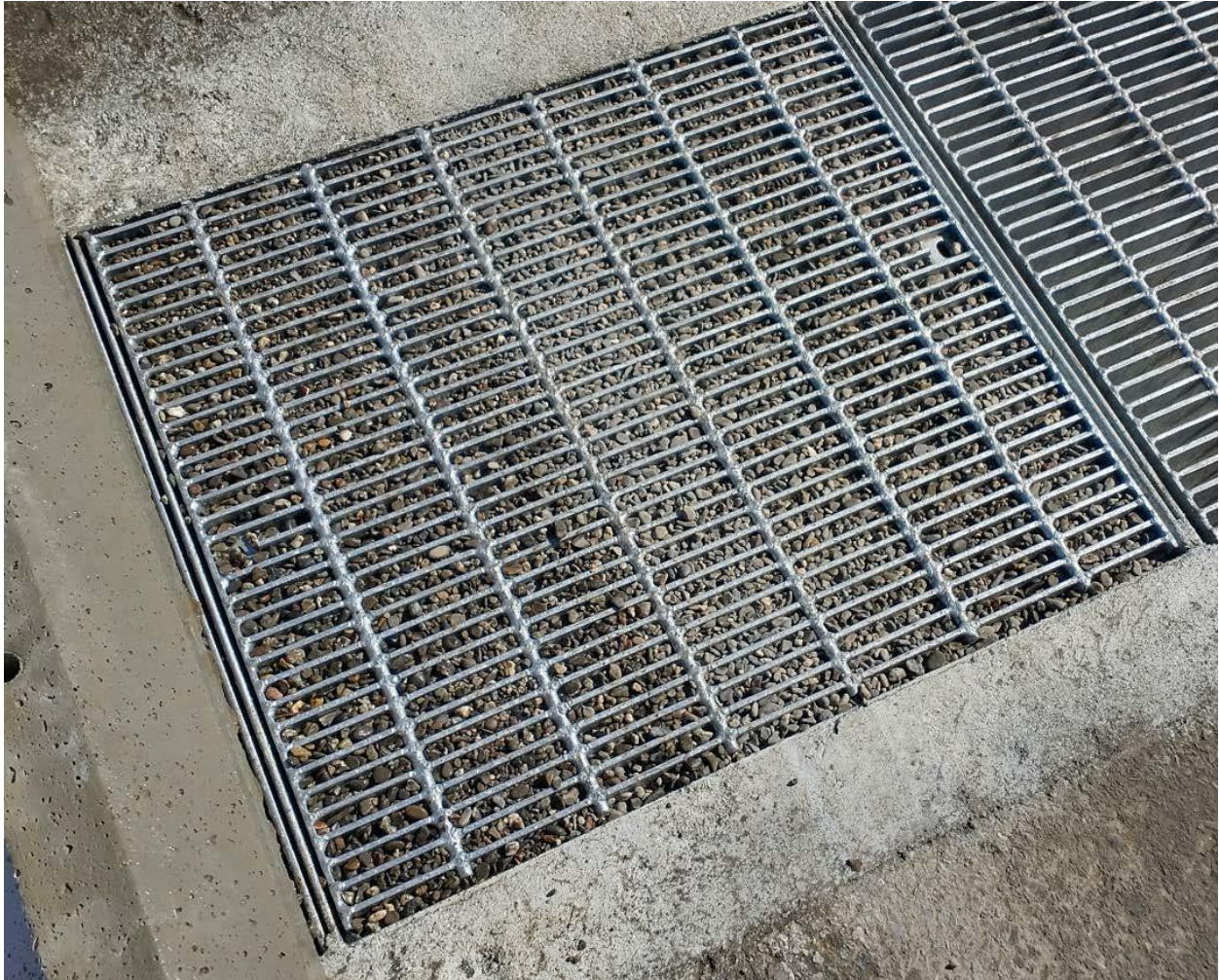
Figure B.2: Test#1 Pass 1 (3/8-inch pea gravel after sweeper pass at normal 2.2 ft/s speed)
