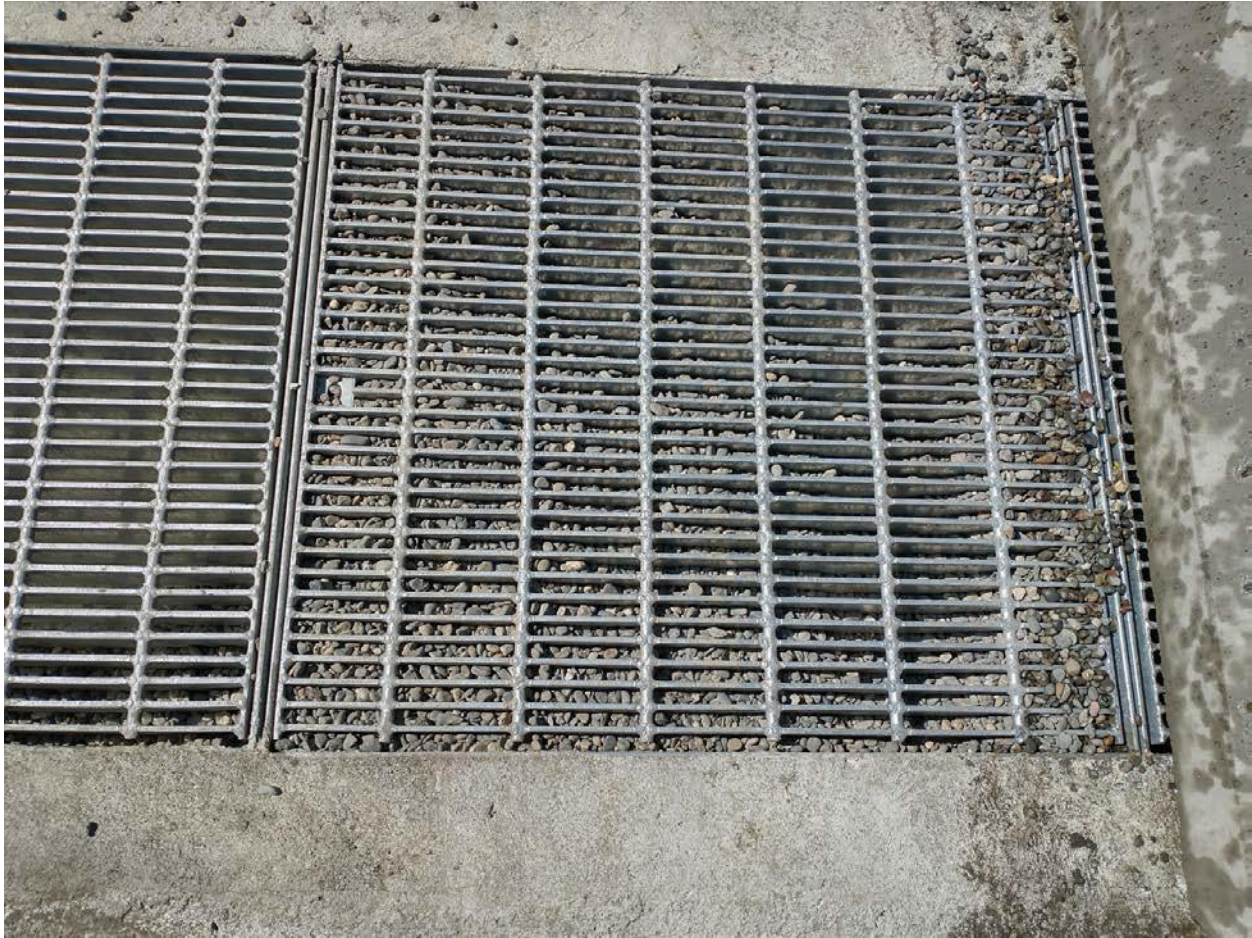
Figure B.4: Test#2 Pass 1 (3/8-inch pea gravel after very slow sweeper pass)
