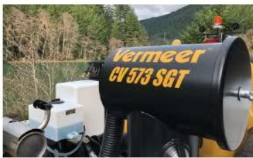
.5 MICRON FILTRATION. Cyclonic filtration separator as well as a secondary filter to clean the air down to .5 microns.
