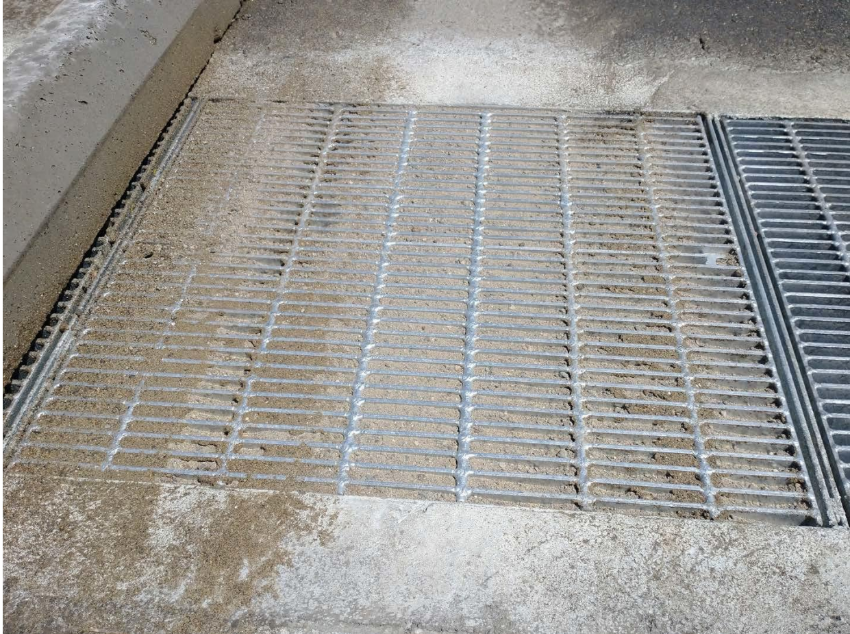
Figure B.5: Test#3 Pass 1 (sand after normal speed sweeper pass at normal 2.2 ft/s speed)
