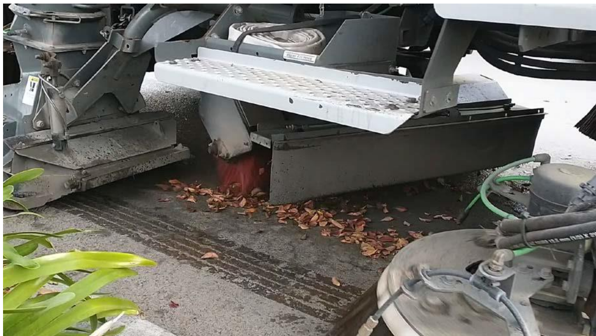
Figure 2.4: Close-up of debris swept toward the pickup head
