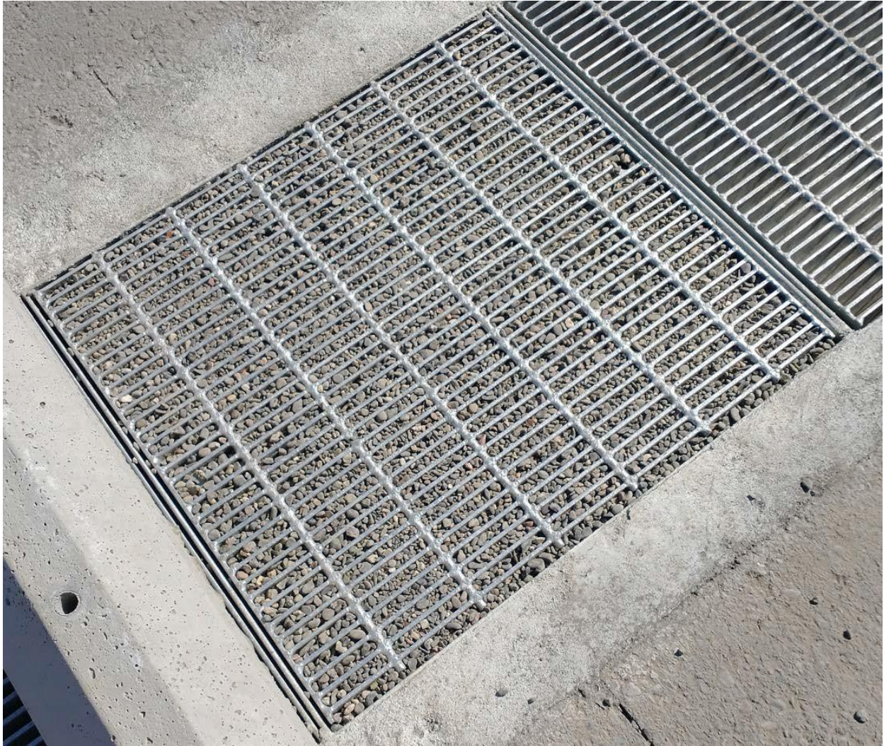
Figure B.1: Test#1 (3/8-inch pea gravel before sweeper pass)
