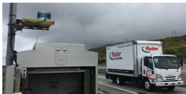
Image 1: A truck is detected and scanned by the Velodyne LiDAR detector as it passes by on the entrance ramp to the San Onofre truck scale beside the Southbound I-5 Freeway.
