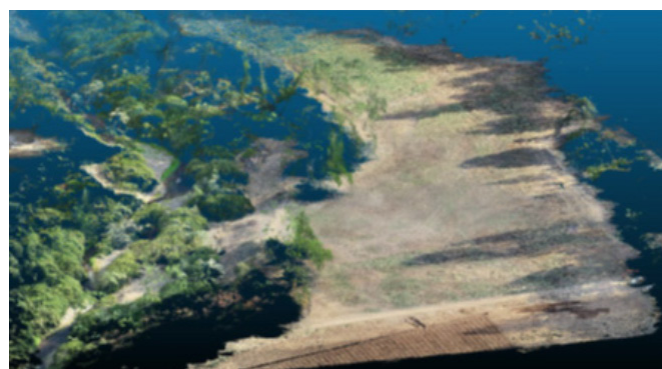
Image 2: Point cloud data generated using Phantom 4 Pro UAS images and WebODM software
