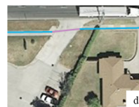
d. section of driveway/parking-lot sidewalk (purple line) is usually the outlet of parking lots or garages. Vehicles pass these sections without signal regulation. Hence there are potential safety hazards and yielding delay for active travelers when they cross these sections.
