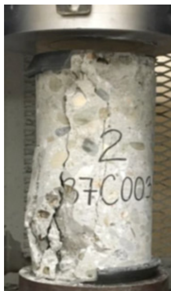
Image 2: Bridge Core after Testing
