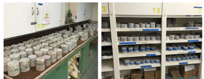
FIGURE 2: Pavement and bridge cores after cutting for visual inspection
