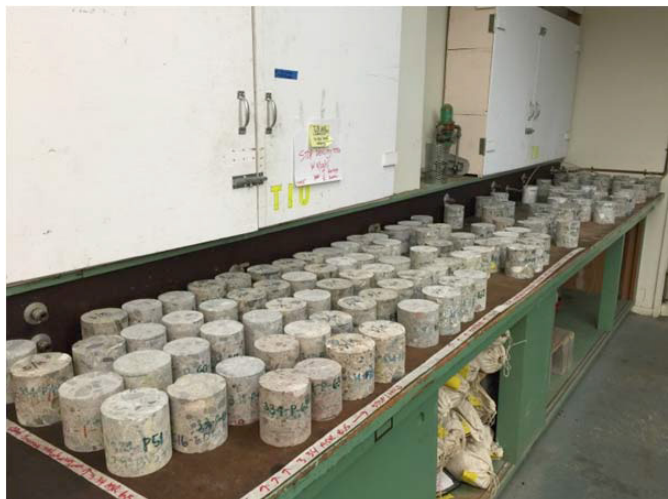
Image 3: Pavement and bridge cores after cutting for visual inspection
