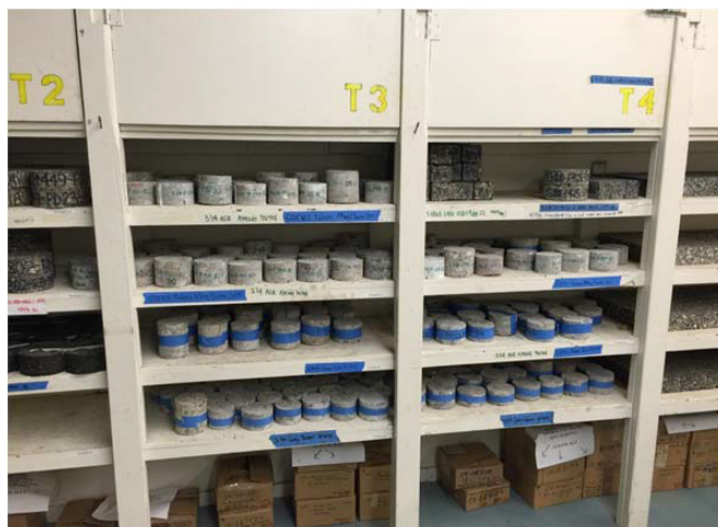
Image 4: Pavement and bridge cores after cutting for visual inspection
