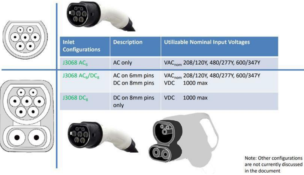
Figure 2.4. Part of Specifications for J3068
