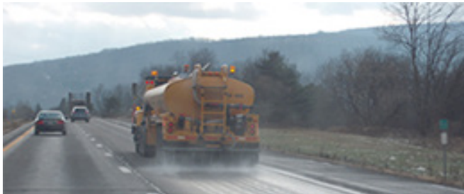
Image 2: Brine tank truck spreading salt brine on roadway
