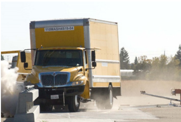
Image 5: Type 85 Bridge Rail: Van Body Impact
