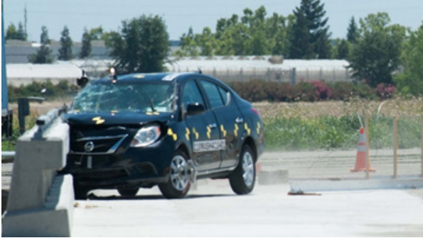
Image 3: Type 85 Bridge Rail: Small Car Impact
