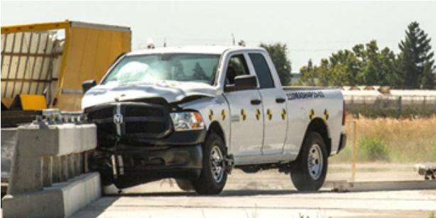
Image 4: Type 85 Bridge Rail: Pickup Truck Impact
