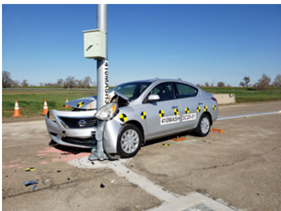
Image 4: TEST 410MASH3C20-01 Small Car 19 MPH Impact (February 26, 2020)
