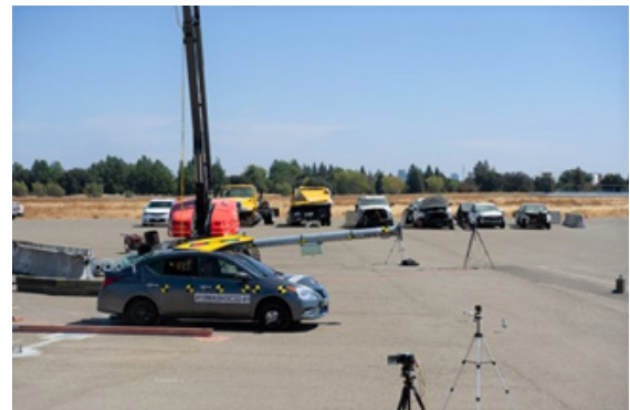
Image 6: TEST 410MASH3C22-01 Small Car 19 MPH Impact (September 14, 2022)
