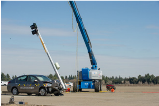
Image 3: Test 430MASH3C17-01 Small Car 31 MPH Impact (March 7, 2018)
