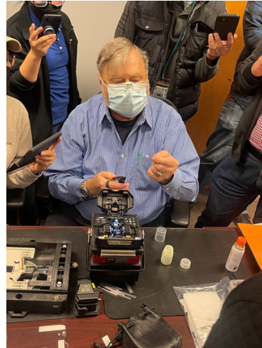
Image 2: Hands-On Fiber Optic Training – Fusion Splicing
