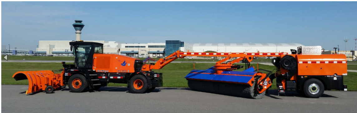
Figure 6. Northstar's Automated Runway Snowplow Machine
